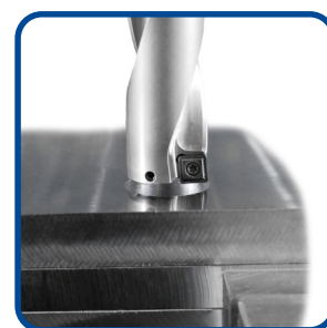
Paketbohren Bundle drilling
